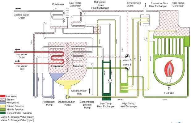
Double-Effect Direct Fired Absorption Chiller & Heater - Normal Efficiency Model (KDA) - COP : 1.18
