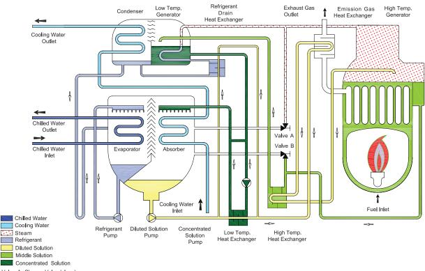
Valve A: Change Valve (close) Valve B: Change Valve (close)
